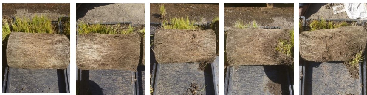
1: 100% soil (zero rice husk) 2: 95% soil (5% rice husk) 3: 90% soil (10% rice husk) 4: 85% soil (15% rice husk) 5: 80% soil (20% rice husk)
