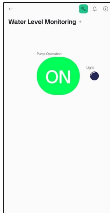
Fig. 6: Manual control through the Blynk application
